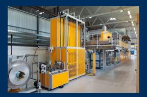
The flexible, customer-specific integration of single or multiple sensor solutions of the SITA clean line CI is used in production processes for the inspection of the smallest parts of medical technology as well as band surfaces in the steel industry.  ✓ Detection of filmic contamination: contact less, non-destructive, layer thickness sensitive
